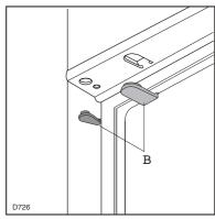
Position the runners (A) at the top and bottom of the inside of the kitchen unit as shown in the diagram and mark the position of the external holes. After preparing the holes, screw the runners to the kitchen unit door using 3.5x16 mm screws.
